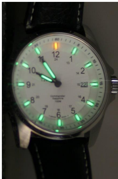
A watch (Swiss, of course) that uses tritium radioluminescence to illuminate the hands [I, Autopilot, CC BY-SA 3.0 via Wikimedia Commons].
